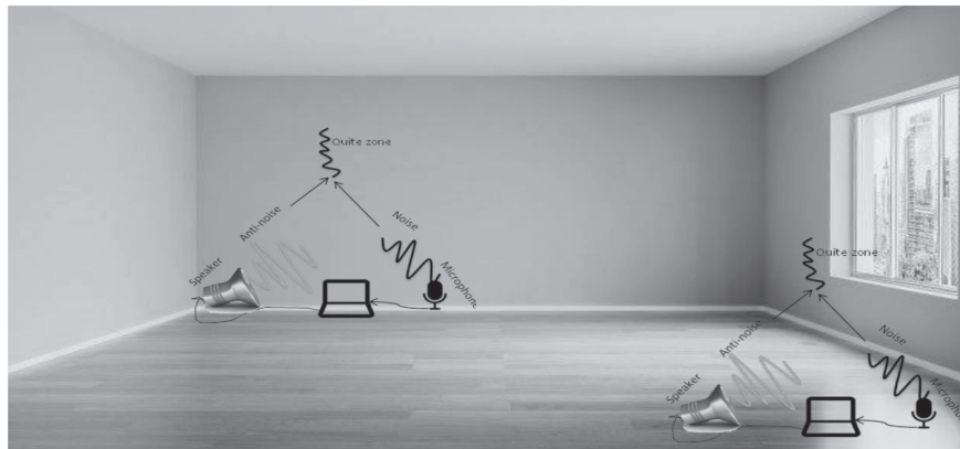
Figure 8: Feedback ANC system inside a room
