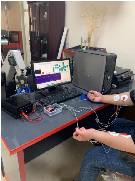
Fig. (2) measuring system for EMG signals of the LH &RH.
