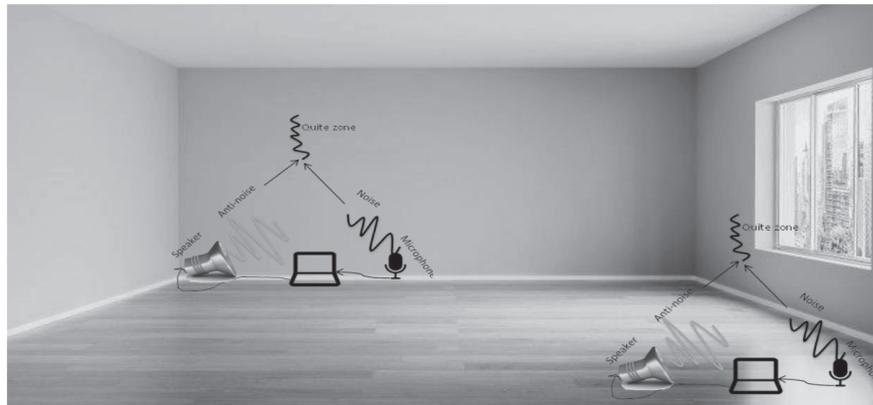
Figure 8: Feedback ANC system inside a room
